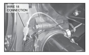
Figure 45. Wire 18 Connection 8 kW Units
